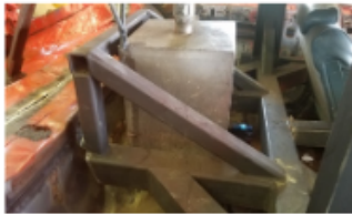
Sample Gas tank protector: Note ALL components must be 4" from sheet metal.
