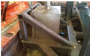
Sample Gas tank protector: Note ALL components must be 4" from sheet metal.
